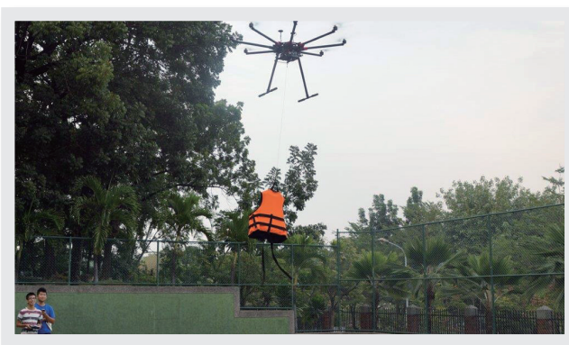
▲ Test fly of unmanned airplane with life jacket hanging.
